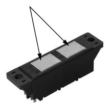
Before mounting, inspect the module to insure that the contact surface of the bottom substrate is clean and free of any lumps or bulges that could damage the device or impede heat transfer across its surface.
